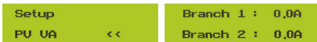
Pic 8.16 PV String current
