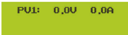
Pic 8.3 PV input voltage and current information
