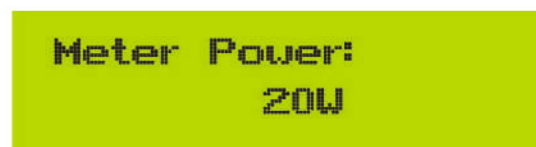
Pic 7.5 Zero-export function via energy meter turn on
