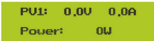
Pic 8.3 PV input voltage and current information
